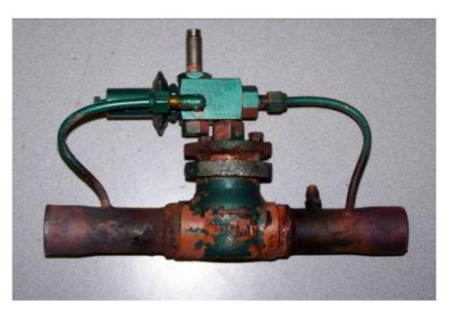
The longer the life of the equipment, the more we will face leaks through deterioration. Valves and other components are constantly in contact with water due to condensation. This creates rust which may potentially evolve into leaks.
