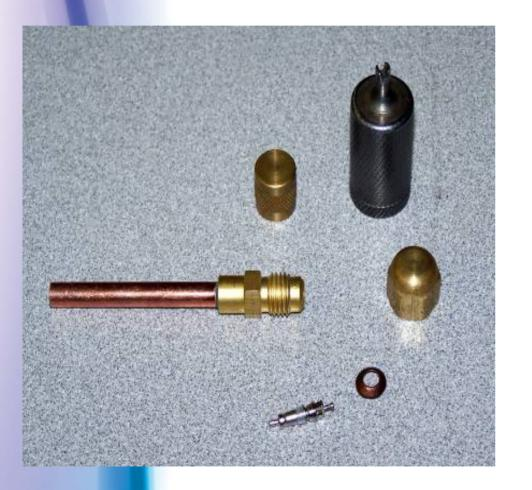
Schrader Valves along with their cores and caps are an entry point as well as sometimes an exit point for refrigerants. It is important to ensure that the valve was not leaking with the core installed and that the core is tight and the proper caps were used. For example, hard caps should be used with a copper gasket for high pressures.
